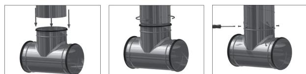
Size and number of screws depending on the diameter of the smoke extraction duct:
