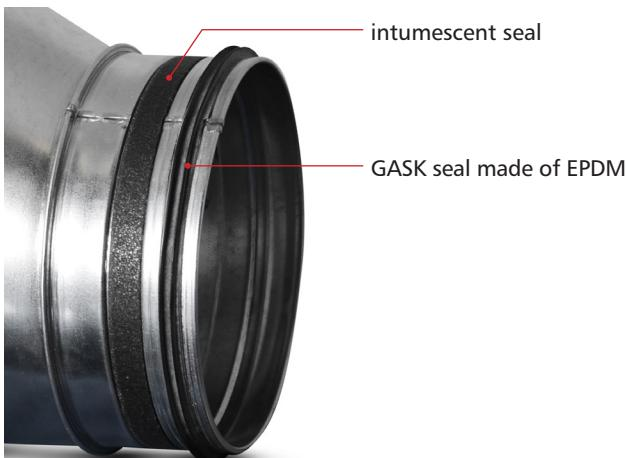
The GASK seal is made of EPDM material, which is resistant to ozone, UV radiation and temperature fluctuations in the range of -30% °C÷+100°C. It is fastened at the end of the male smoke extraction coupling through its rolled-up, tightened edge.
