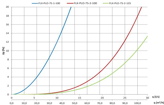
Pressure drop diagram for an exhaust plenum box: Ø100, Ø125
