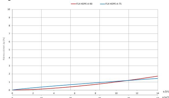
\* greater pressure drop for higher airflow for 90mm duct occurs because of its curved inner structure
