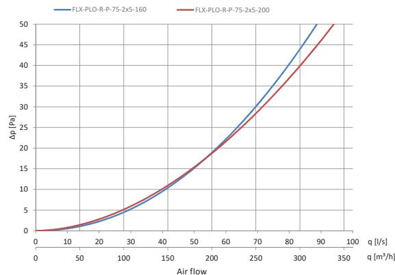
Silencer for heat recovery ventilation system
