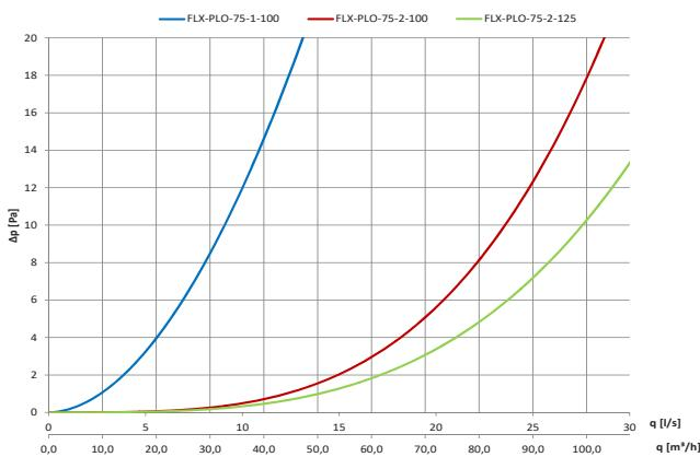
Pressure drop charts for the exhaust air plenum box: Ø100, Ø125
