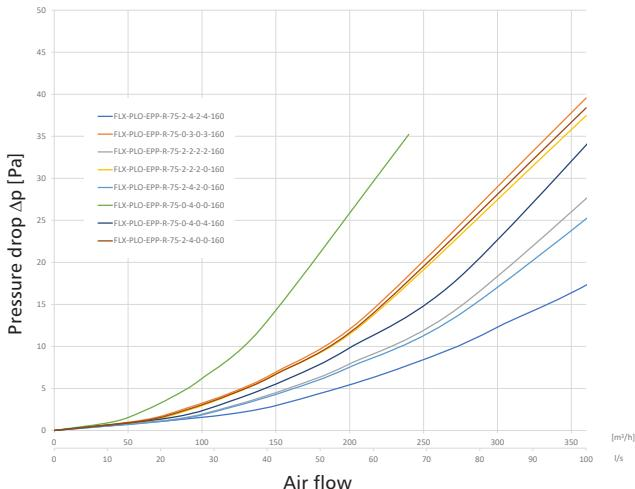
Pressure drop chart (supply air) for manifolds up to 18 spigots
